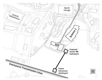
This project establishes a second connection to Eversource, terminating at a new 50-75 MVA transformer located on the exterior of the Supplemental Utility Plant (SUP) in the substation switchgear yard. Included is a required modernization of the electrical distribution control system to manage multiple sources and the increased load demands which enables code compliant switching for personnel safety. The project is currently in the Design phase with expected construction start in 2026.
